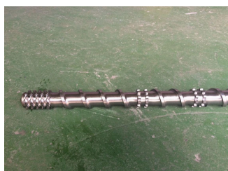
Nitrided alloy steel screw
