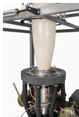
Die head and double-lip air ring
