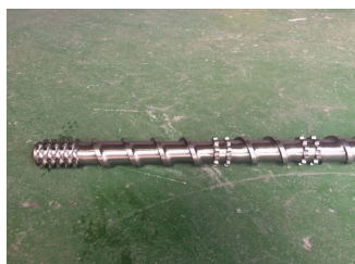
Nitrided alloy steel screw
