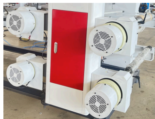
Double unwinder and double rewinder
