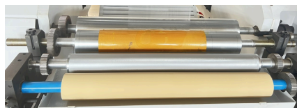
Corrosion resistant rubber roller
