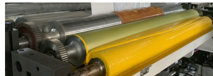
Rubber roller, anilox roller and printing cylinder
