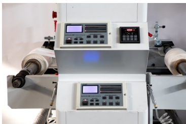
Automatic tension and web-guide controls
