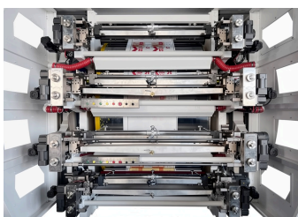
Printing units arranged around the central impression drum
