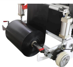
Unwinder with magnetic brake and air shaft
