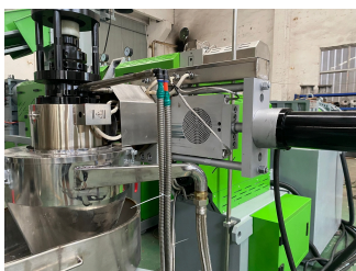
Second hydraulic screen changer and die head
