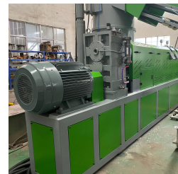
First-stage extruder — motor and gearbox
