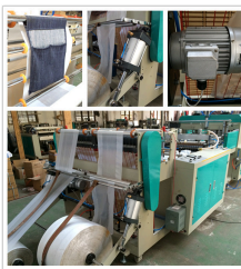
Unwinding — air-cylinder roll loading and inverter-controlled unwind
