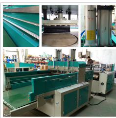
Punching unit and PU conveyor
